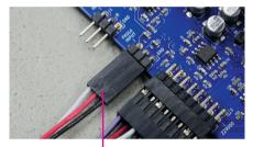
Connect **one end** of the Internal Audio Cable to the PAULA INPUT header on ZZ9000AX as pictured.
