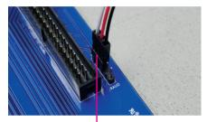
Connect the **other end** of the Internal Audio Cable to the AAUD header on ZZ9000 as pictured. The 2 pins close to the AAUD label are left open.
