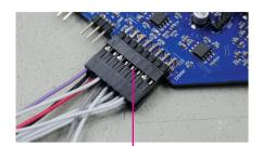
Connect the **second half (8 pins, only 1 purple and 2 white leads)** of Data Cable to the **top row** of ZZ9000 header on ZZ9000AX as pictured.
