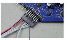
Connect the **first half (8 pins, black/ red/gray/white)** of the Data Cable to the **bottom row** of ZZ9000 header on ZZ9000AX as pictured.
