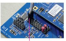
Connect **white and gray leads** to the **second column** of the MIO header on ZZ9000. Make sure to skip the first two pins of the header!
