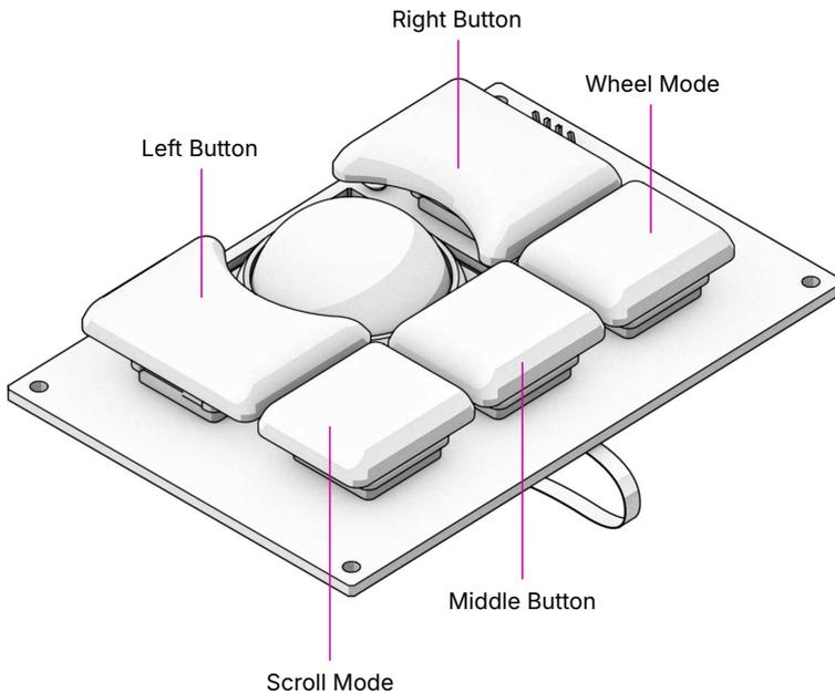
The trackball works like a mouse with three buttons (left,
