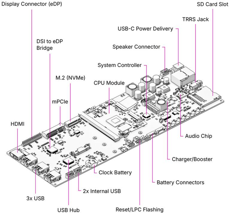
The Motherboard spans the inner width of the device and has outward-facing ports on both sides. It is mounted to the Main Box with four M2×4 pan head screws. The Motherboard has the following main features:
