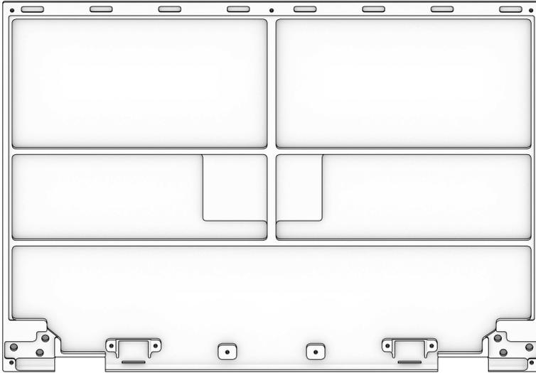
The eDP display panel rests in the Screen Back. The left and right hinges are mounted in the bottom left and right corners with three M4×5 countersunk screws each. Note that the hinge labeled “SMS-ZZ-219-L” goes on the right side, and the hinge labeled “SMS-ZZ-219-R” goes on the left side. The other half of each hinge is mounted to the Main Box with four M2×6 countersunk screws.
