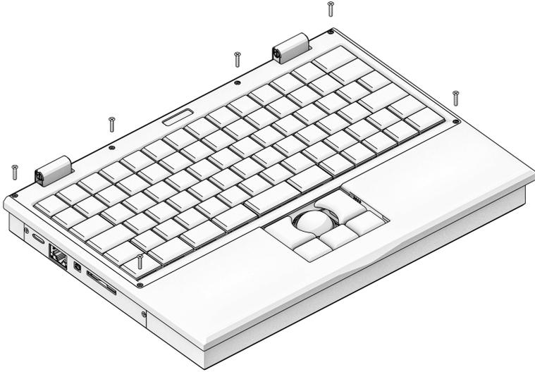
The Keyboard Frame is inserted into the Main Box. It has four tabs on the front that must be inserted first. The frame is mounted with six black M2×5 countersunk screws.
