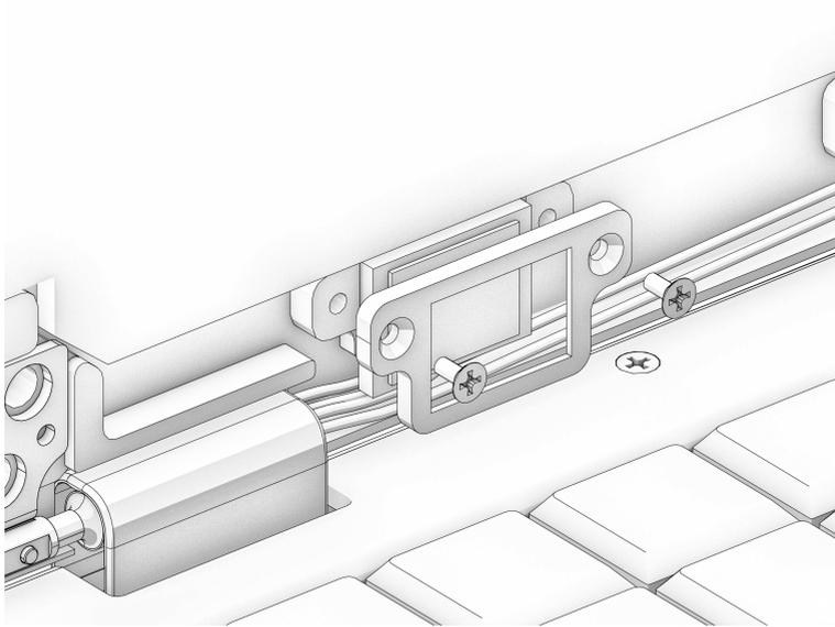
The stereo speakers are mounted below the display and secured with the speaker holders. Each holder is mounted with two black M2×5 countersunk screws. Both speaker and display cable are fed through a cutout in the hinge and into the Main Box.
