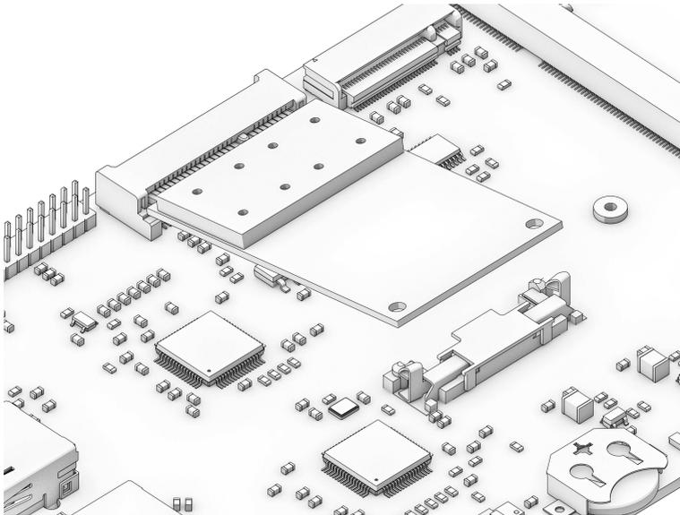
All Processor Modules feature at least one PCIe controller which is connected to the mPCIe socket U11. The standard use for the mPCIe port is a WiFi card or an NVMe SSD (with M.2 adapter). To install a card, plug it into the socket at an
