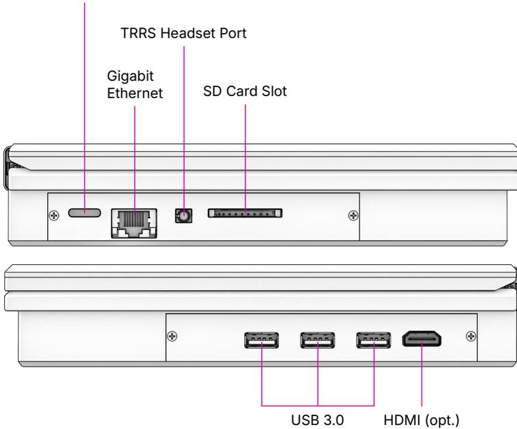
The Port Covers are two pieces of powder coated steel that cover the side openings of the Main Box (mounted with two black M2×5 screws each). You can exchange these to fit a future motherboard or an expansion that requires a different port layout.
