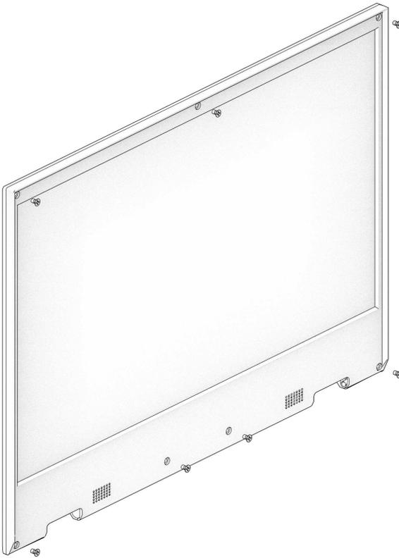
This part serves as a bezel for the display. It is mounted with seven black M2×5 countersunk screws to the Screen Back.
