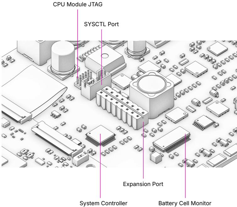
The Expansion Port U18, labeled “Hack the Planet” is meant for advanced users that want to connect sensors or other peripherals to MNT Reform’s system controller. Please note that changing the system controller’s program can disrupt the battery charging control loop, potentially causing over- or undercharged cells, resulting in physical damage and/or injury. **Experiment with the system controller only if you know exactly what you’re doing and at your own risk.**
