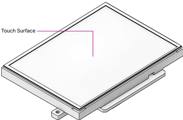
Unlike the trackball, the trackpad doesn't have any buttons. Slide one finger across the surface to move the cursor. Tapping with one finger acts like a left mouse button click. Slide two fingers across the surface to scroll in any direction. Tapping with two fingers performs a right click. To click and drag, use three fingers. Tapping with three fingers is equivalent to a middle click.
