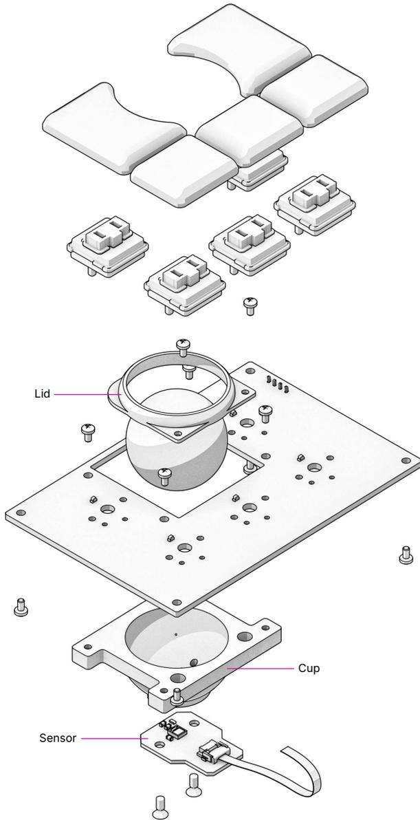
The trackball uses an RP2040 microcontroller to convert X and Y movement coordinates from the PAT9125EL optical sensor that is connected via I<sup>2</sup>C to the USB HID Mouse protocol. The electronic connection between trackball sensor and controller is made with a 6-pin 0.5mm pitch flex cable.
