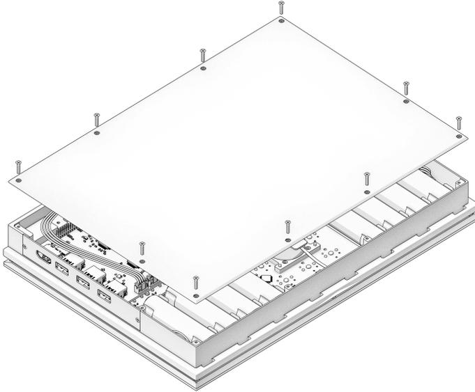
The Bottom Plate closes the Main Box from the bottom with ten M2×6 countersunk screws.
