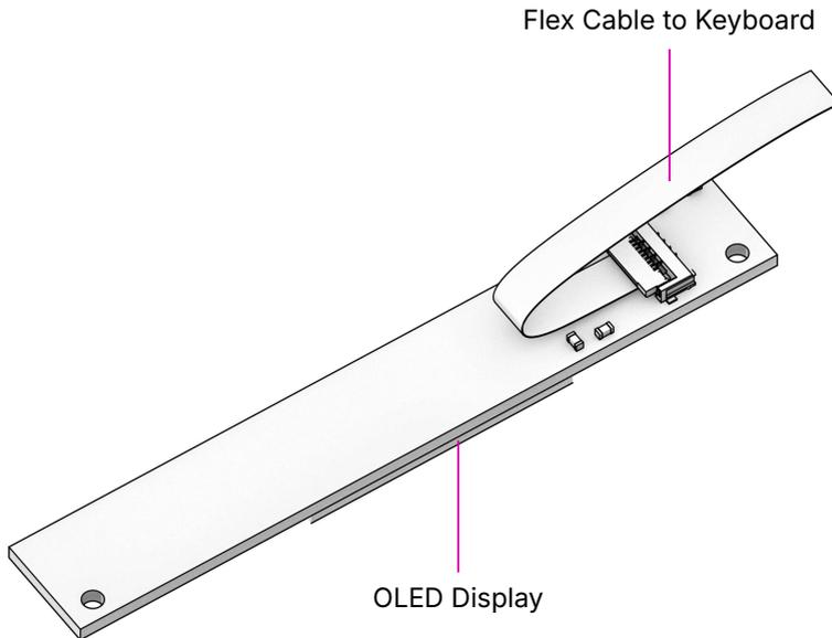
The OLED display sits on the OLED Module which is connected to the keyboard through a 4-pin, 1mm pitch flex cable. The communication protocol is I<sup>2</sup>C. The module is mounted in the Main Box on top of the keyboard with two M2×4 pan head screws.
