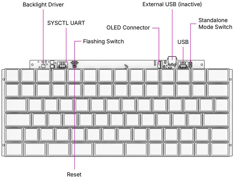
The keyboard is mounted to the top of the Main Box with six M2×4 pan head screws. It is powered by an RP2040 microcontroller. The controller scans the row/column matrix of keyswitches and reports key presses via USB HID (human interface device) to the motherboard. Each switch has a diode to prevent ghosting, so you can press multiple keys at once. The microcontroller runs a firmware based on `pico-sdk` and `tinyusb` which is an open source library for implementing USB input devices.
