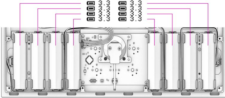
The illustration shows which icon and voltage on the OLED display corresponds to which battery cell in the device.<sup>2</sup>
