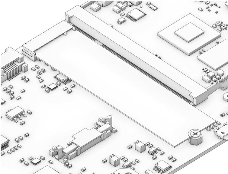
Some Processor Modules, such as the original i.MX8M module and the RCORE with RK3588, feature a second PCIe controller—or in the case of LS1028A, a SATA controller—which is connected to the M.2 socket (J10). The standard use for the port is to install an M.2 NVMe solid state drive. Plug the SSD disk into the socket and fix it with an M2 screw to one of the three mounting holes that corresponds to the module's size.
