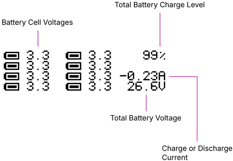
You can see detailed battery information including the estimated total charge percentage on the Battery Status screen reachable through the OLED menu. Each cell icon corresponds to one of the eight battery cells. The leftmost group of four icons represents the battery pack on the left side of the device, and the group on the right represents the battery pack on the right—assuming you look at MNT Reform when flipped on its back and the batteries closest to you.
