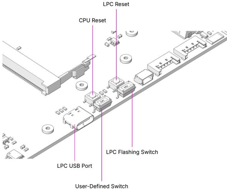
To update (flash) the firmware of the System Controller, you need another computer and a USB-C cable (or, if you have a motherboard older than version 2.5, a Micro-USB cable).
