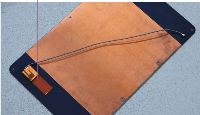
Secondary antenna placement
