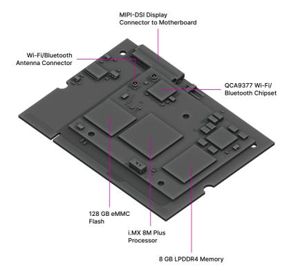
The first version of the MNT Pocket Reform ships with an NXP i.MX8M Plus Processor Module. We are constantly developing new modules for Pocket Reform with different features to accommodate individual preferences, like the fast and cost-effective RCM4-BPI module with Amlogic A311D or the latest drop, RCORE with RK3588—a powerful Processor Module that gives you 4x performant ARM Cortex-A76 cores, 4x power-efficient ARM Cortex-A55 cores, and up to 32 GB RAM.
