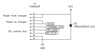
"Raw power" from an external source—in this case, from a USB-PD charger—enters the charging board, and system power, sourced and regulated by the MPS from either the batteries or the external input, comes out and goes back to the motherboard. The I2C bus is for communication with the charger and protector chips.
