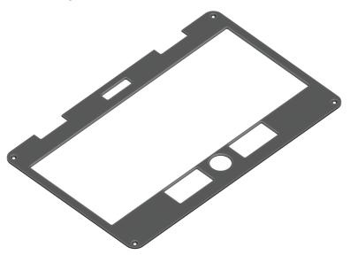
The keyboard frame is a 1.2 mm thick anodized milled aluminum plate that acts as the bezel for the keyboard, trackball, and the OLED display. It is attached with 4 M2 screws.
