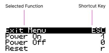
The keyboard has a built-in OLED display for interaction with the System Controller on the motherboard. You can highlight an option and scroll through the menu by using the  $\uparrow$  and  $\downarrow$  keys. To trigger the highlighted option, press *ENTER*. Alternatively, you can press the shortcut key that is displayed on the right hand side of each menu option. For example, to show the Battery Status, press B when the menu is active. To leave the menu, press ESC.
