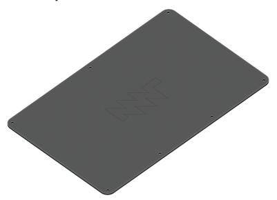
The top back cover is a 1.2 mm PCB that covers the motherboard. There is a large exposed copper area in the middle of the cover. It serves as the heatsink and has to be thermally attached to the CPU processor module using a square of a 2 mm thick thermal pad. It is attached with 7 M2 screws.
