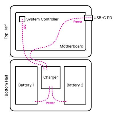
Underneath the keyboard reside two LiPo battery cells with 606090 form factor. In their middle: the charger board. This little PCB mainly contains two chips: one is a fuel gauge with battery protection (MAX17320G20+), and one is the actual charger, the MPS MP2762A. These chips are decoupled from the motherboard to allow for future flexibility in terms of battery architectures and chemistries, and to allow both the motherboard and the charger to be reused in other contexts.
