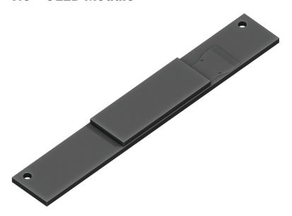
The OLED display sits on the OLED Module which is connected to the keyboard through a 4-pin, 1 mm pitch flex cable. The communication protocol is  $I^2C$ . The module is mounted in the Main Box on top of the keyboard with two  $M2\times4$  pan head screws.
