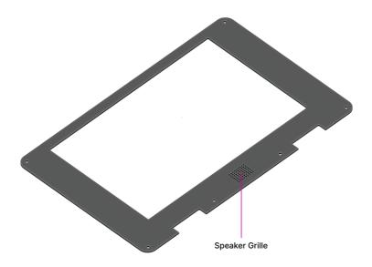
The display frame is a 1.2 mm PCB and acts as a bezel for the display and the speaker. It is attached with 6 M2 screws.
