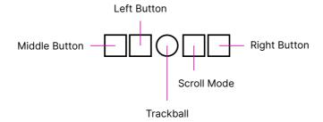
The trackball works like a mouse with four buttons: middle button, left click, scroll button, and right click. Roll the ball to move the cursor. Pressing the *Middle Button* and the *Scroll Mode* button simultaneously activates *Sticky Scroll Mode*, so
