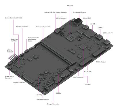
The Motherboard spans the inner width of the device and has outward-facing ports on both sides. It is mounted to the Main Box with two M2×3.5 and two M2×5 countersunk screws. The Motherboard has the following main features:
