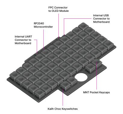
The keyboard is mounted to the top of the Bottom Half with six M2×4 pan head screws. It is powered by an RP2040 32-bit microcontroller. The controller scans the row/column matrix of keyswitches and reports key presses via USB HID (human interface device) to the motherboard. Each switch has a diode to prevent ghosting, so you can press multiple
